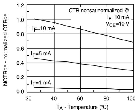
Figure 4. Current Transfer Ratio (normalized) vs. Ambient Temperature
