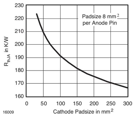
Figure 6. Thermal Resistance Junction Ambient vs. Cathode Padsizes
