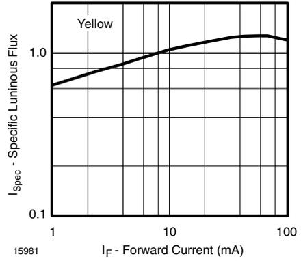
Figure 12. Specific Luminous Flux vs. Forward Current
