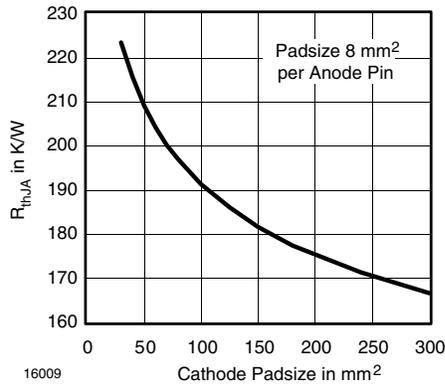
Figure 15. Thermal Resistance Junction Ambient vs. Cathode Padsize
