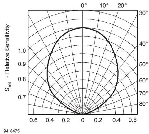
Figure 8. Relative Radiant Sensitivity vs. Angular Displacement
