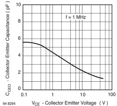
Figure 8. Collector Emitter Capacitance vs. Collector Emitter Voltage
