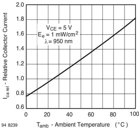
Figure 3. Relative Collector Current vs. Ambient Temperature
