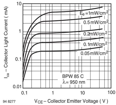
Figure 7. Collector Light Current vs. Collector Emitter Voltage
