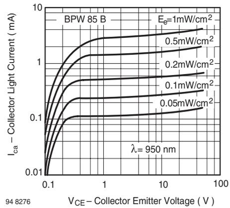
Figure 6. Collector Light Current vs. Collector Emitter Voltage
