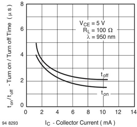
Figure 9. Turn On/Turn Off Time vs. Collector Current
