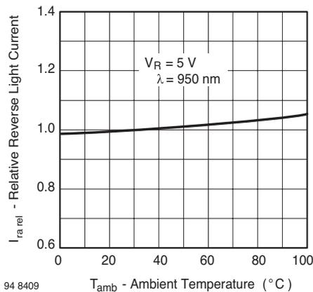
Figure 2. Relative Reverse Light Current vs. Ambient Temperature
