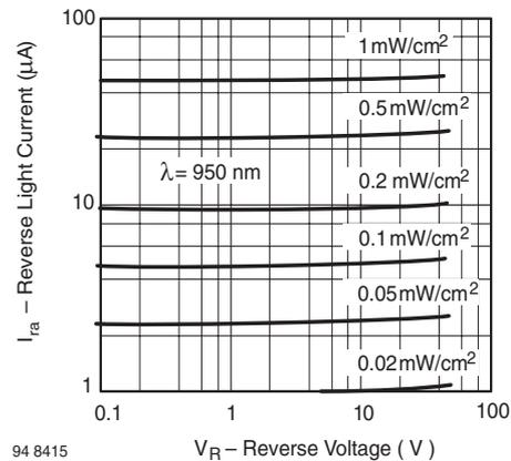
Figure 4. Reverse Light Current vs. Reverse Voltage
