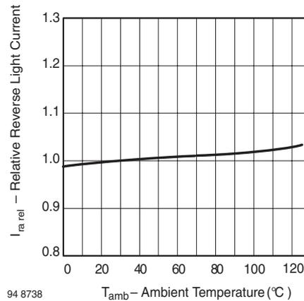
Figure 2. Relative Reverse Light Current vs. Ambient Temperature
