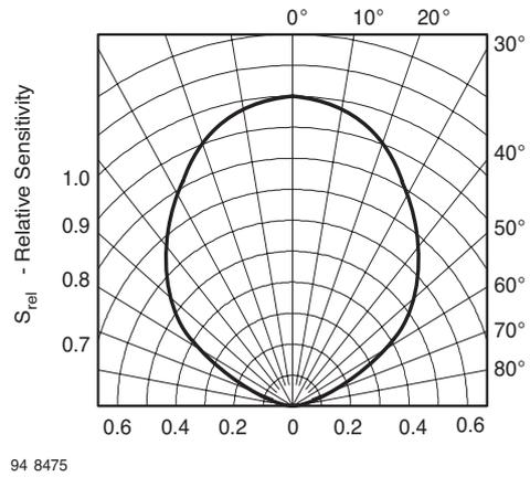
Figure 6. Relative Radiant Sensitivity vs. Angular Displacement
