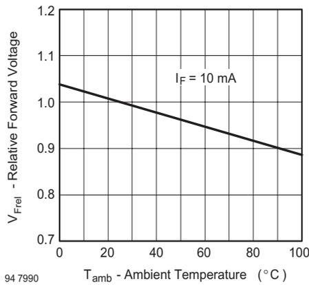
Figure 5. Relative Forward Voltage vs. Ambient Temperature
