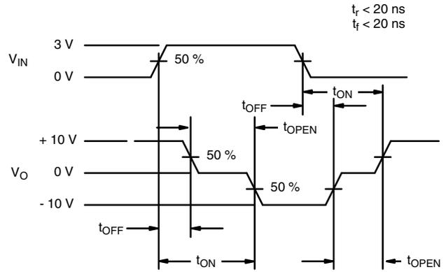
Repeat Test for IN<sub>2</sub>, IN<sub>3</sub> and IN<sub>4</sub>
