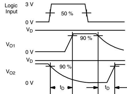
$R_L = 300 \Omega$ ,  $C_L = 35 \text{ pF}$
