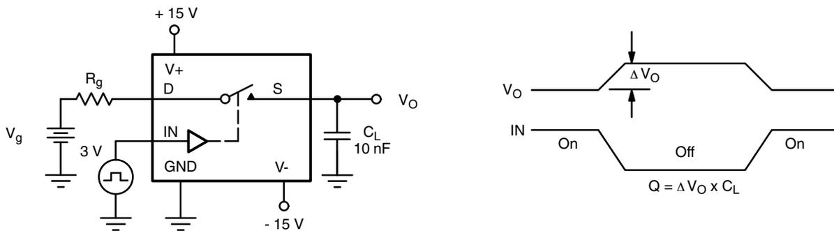
Figure 7. Charge Injection
