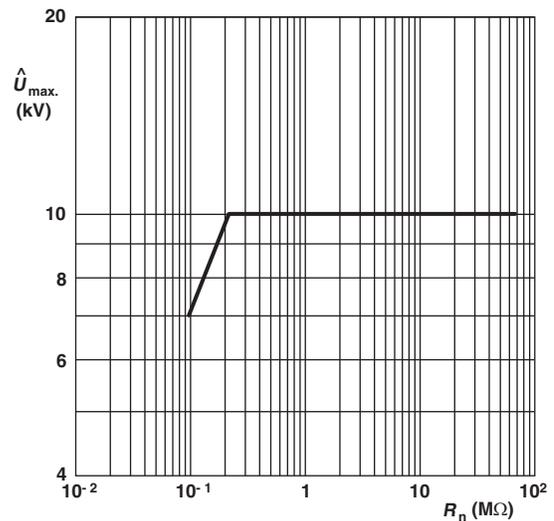
Maximum allowed peak pulse voltage in accordance with IEC 60065, 14.1.a); 50 discharges from a 1 nF capacitor charged to Umax.; 12 discharges/min (drift ΔR/R ≤ 2 %)
