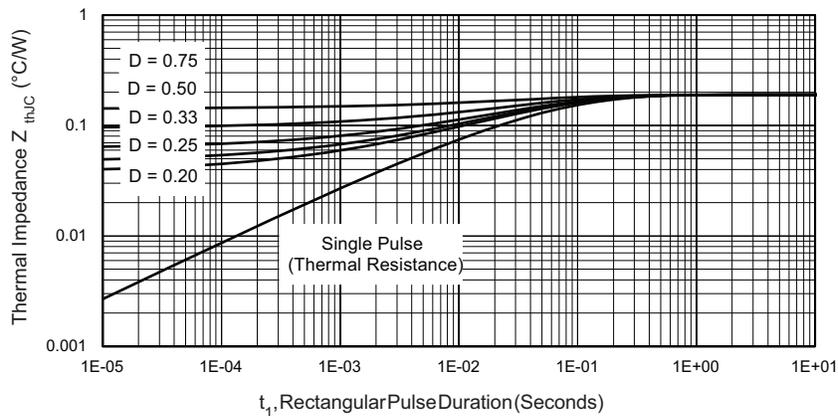
Fig. 4 - Maximum Thermal Impedance  $Z_{thJC}$  Characteristics
