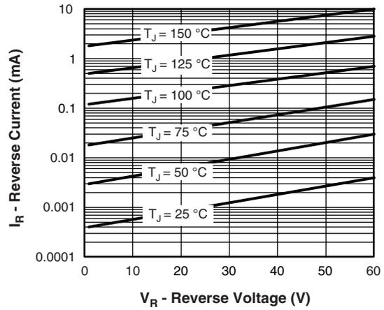
Fig. 2 - Typical Peak Reverse Current vs. Reverse Voltage
