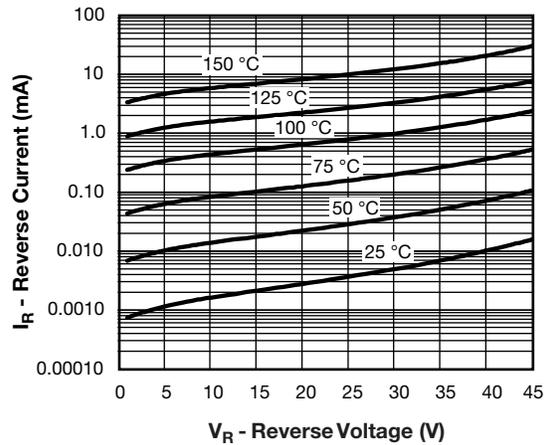
Fig. 2 - Typical Reverse Current vs. Reverse Voltage
