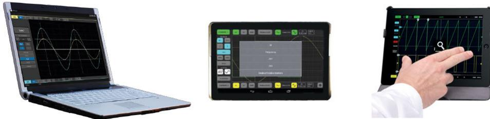
The Velleman **WFS210** is the world's first Wlan dual channel digital storage oscilloscope geared towards tablet computers, it's a compACT, portable, battery powered, fully featured two channel oscilloscope. As opposed to traditional oscilloscopes, it does not feature a screen.
