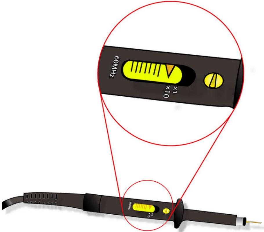
**IMPORTANT: X10 measuring probes should be calibrated.**
