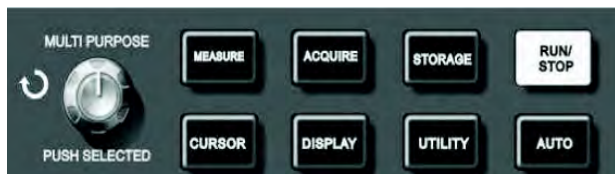
Figure 2—18 Function key of sampling system User can use ACQUIRE key to pop out sampling setup menu so as to adjust sampling mode by control button shown in the menu.
