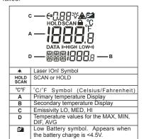
Figure 3. Thermometer Display
