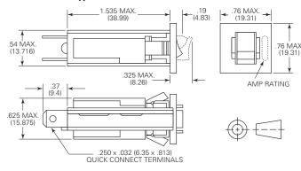
1. Soldering to terminals is not recommended
