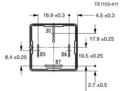
**Power Relay F7/VF7 with PCB Terminals**
