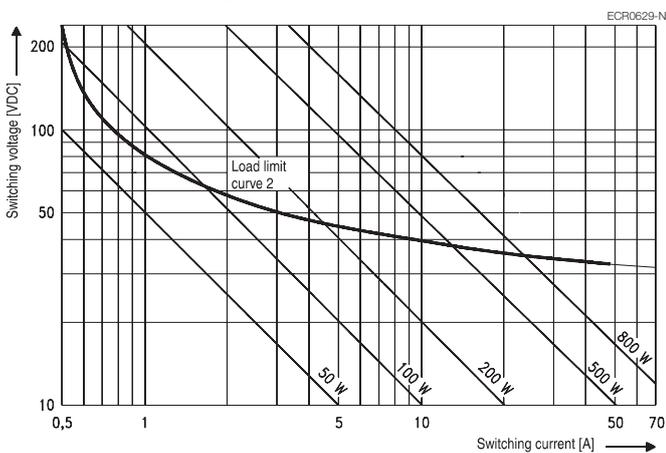
Load limit curve: safe shutdown, no stationary arc/make contact.
