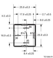
\*) For the make contact (2 x 87), pin 87a = 87 For the double make contact, pin 87a = 87b
