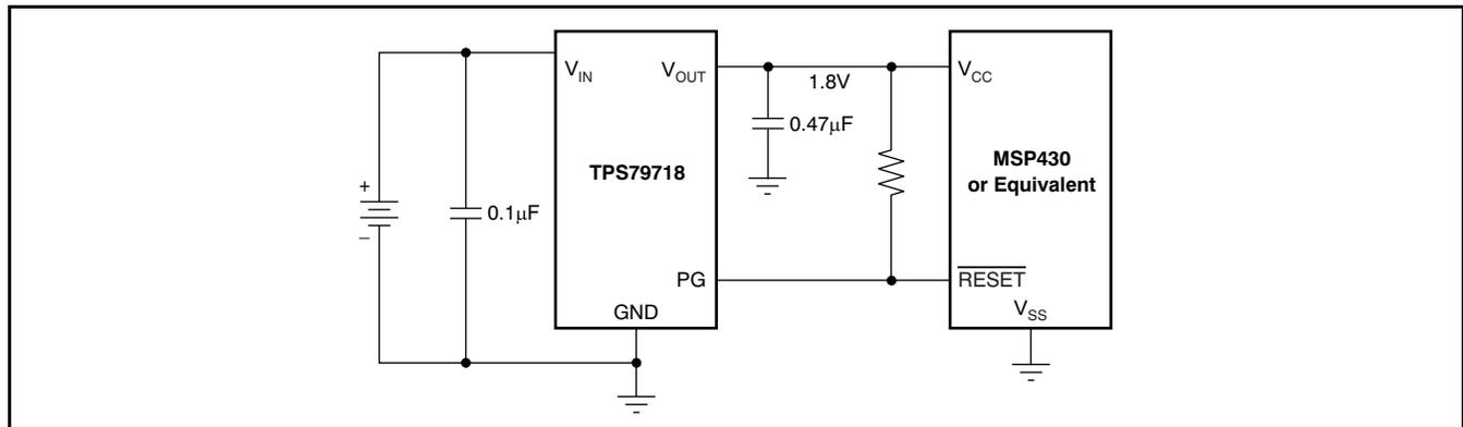
Figure 15. MSP430 Microcontroller Powered by the TPS79718 Regulator
