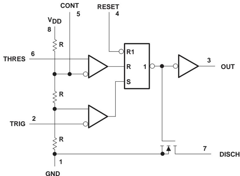
Pin numbers are for all packages except the FK package. RESET can override TRIG, which can override THRES.
