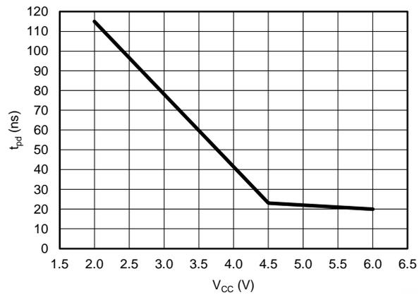
**Figure 5. Propagation Delay vs Supply Voltage at T<sub>A</sub> = 25°C**
