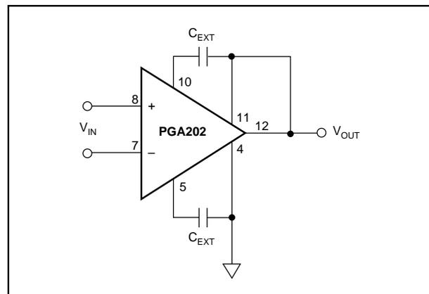
FIGURE 5. Output Filtering.
