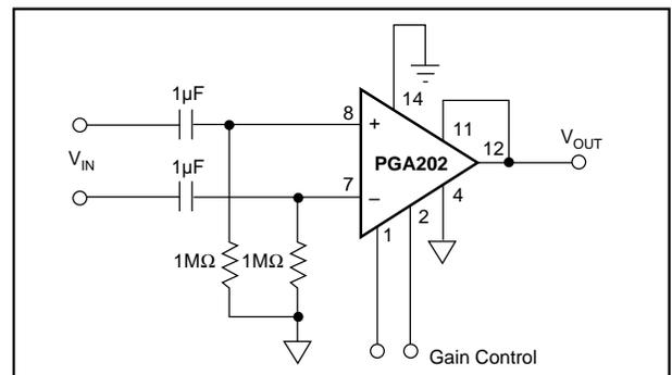
FIGURE 8. AC-Coupled Differential Amplifier for Frequencies Above 0.16Hz.
