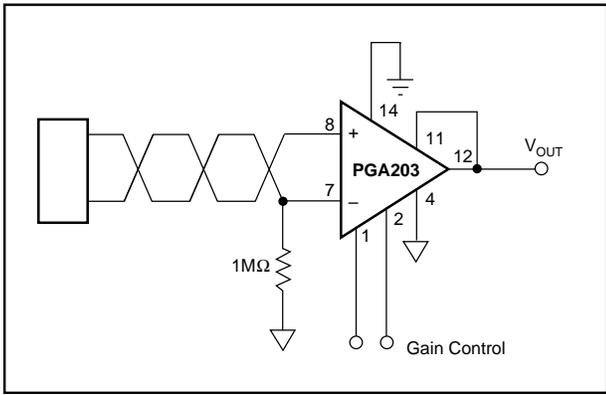
FIGURE 9. Floating Source Programmable Gain Instrumentation Amplifier.
