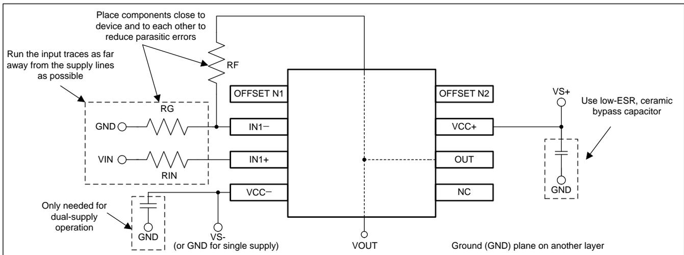
Figure 8. Operational Amplifier Board Layout for Noninverting Configuration
