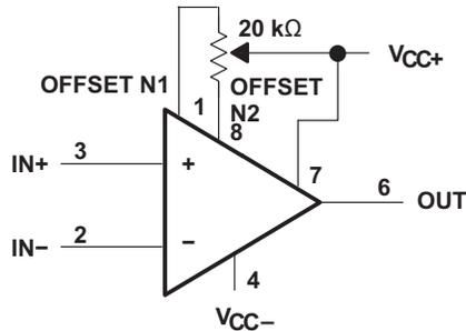
**Figure 2. Input Offset-Voltage Null Circuit**
