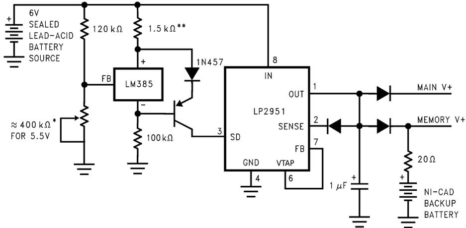
For values shown, regulator shuts down when  $V_{in} < 5.5$  V and turns on again at 6 V. Current drain in disconnected mode is approximately 150  $\mu$ A.
