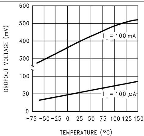
Figure 11. Dropout Voltage
