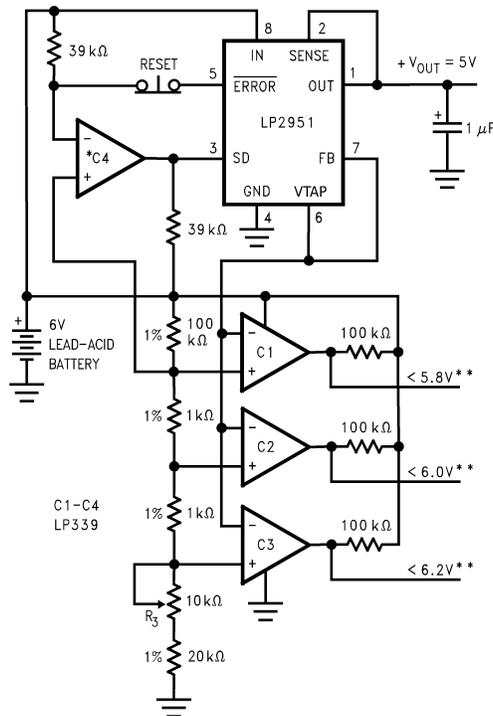
\*Optional latch off when drop out occurs. Adjust R3 for C2 Switching when  $V_{in}$  is 6 V.
