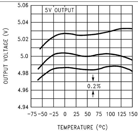
Figure 5. Output Voltage vs. Temperature of 3 Representative Units
