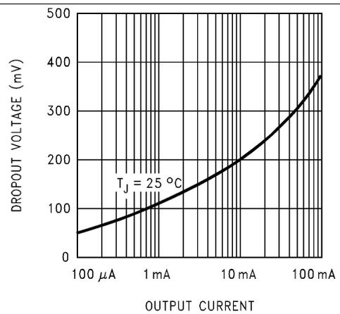
Figure 12. Dropout Voltage
