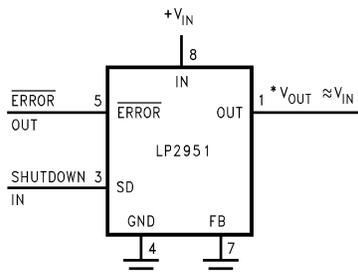
\*Minimum input-output voltage ranges from 40 mV to 400 mV, depending on load current. Current limit is typically 160 mA.
