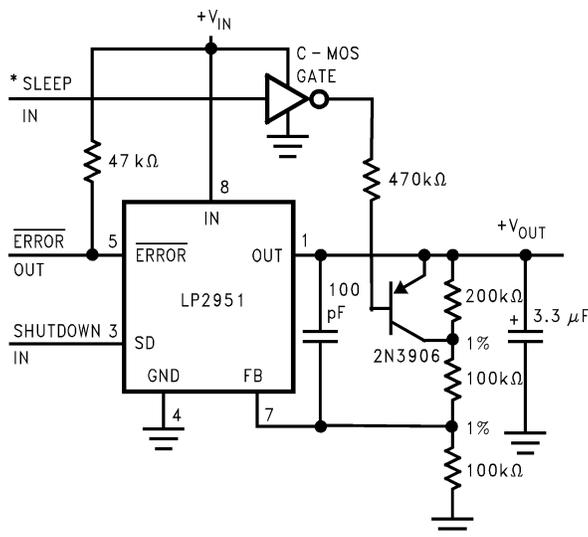
\*High input lowers  $V_{out}$  to 2.5 V.
