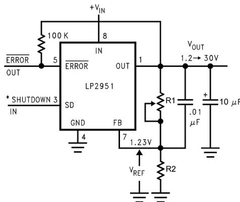
$$V_{out} = V_{Ref} \left( 1 + \frac{R_1}{R_2} \right)$$
