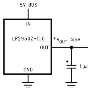
\*Minimum input-output voltage ranges from 40 mV to 400 mV, depending on load current. Current limit is typically 160 mA.
