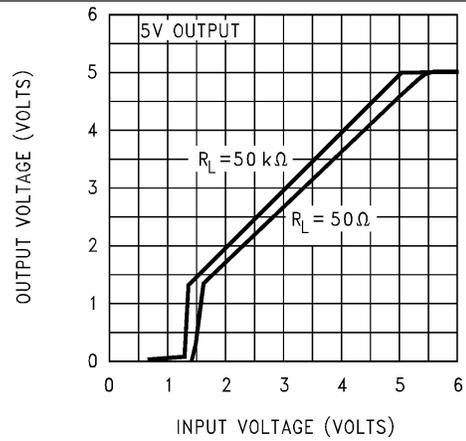
Figure 2. Dropout Characteristics
