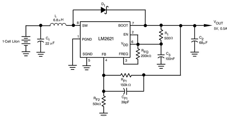
**Figure 13. Typical Circuit**
