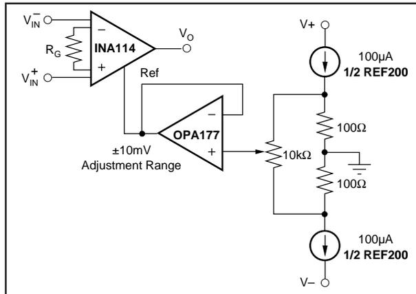
FIGURE 2. Optional Trimming of Output Offset Voltage.
