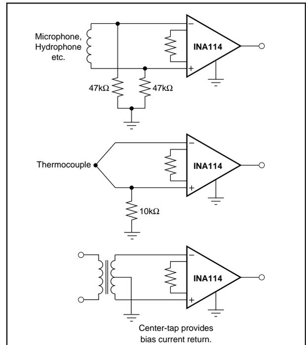
FIGURE 3. Providing an Input Common-Mode Current Path.
