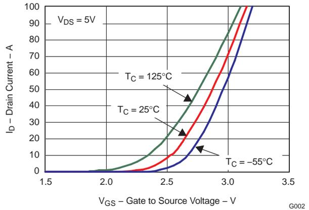
**Figure 3. Transfer Characteristics**
