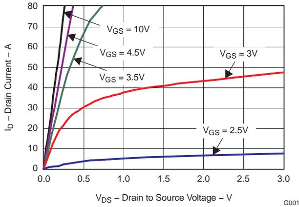
**Figure 2. Saturation Characteristics**
