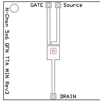
Max  $R_{\theta JA} = 118^{\circ}\text{C/W}$
