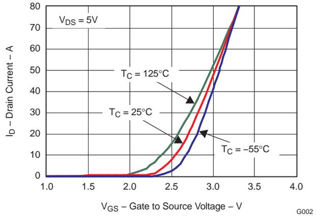
**Figure 3. Transfer Characteristics**
