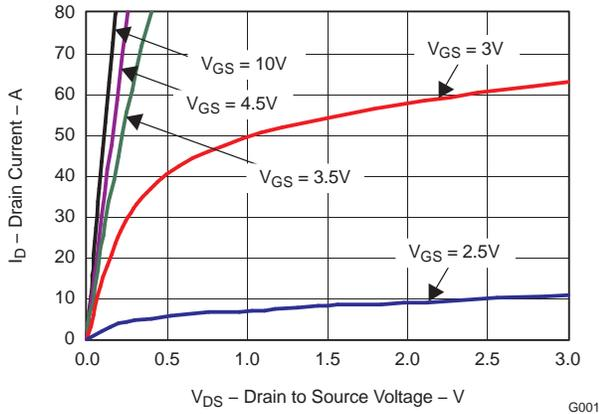
**Figure 2. Saturation Characteristics**
