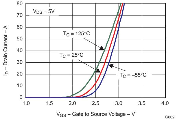
**Figure 3. Transfer Characteristics**
