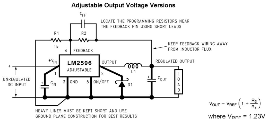
$C_{in} = 470\mu F, 50V, C_{out} = 220\mu F, 35V$  (Aluminum Electrolytic Nichicon "PL Series")
