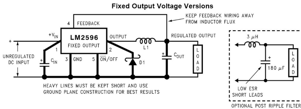
$C_{IN} = 470\mu F, 50V, C_{OUT} = 220\mu F, 25V$  (Aluminum Electrolytic Nichicon "PL Series")
