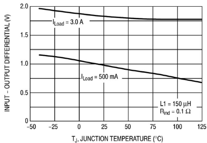
**Figure 4. Dropout Voltage**
