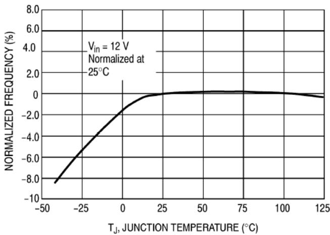
**Figure 10. Oscillator Frequency**
