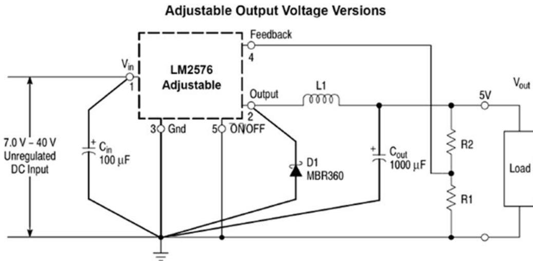
$$V_{out} = V_{ref} \left( 1.0 + \frac{R2}{R1} \right)$$
