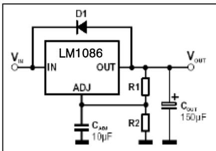
Unlike older regulators, the LM1086 family does not need any protection diodes between the adjustment pin and the output and from the output tu the input to prevent over-stressing the di. Internal resistors are limiting the internal current paths on the LM1086 adjustment pin, therefore even with capacitors on the adjustment pin no protection diode is needed to ensure device safety under short-circuit conditions.
