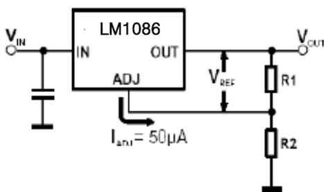
The LM1086 series develops a 1.25V reference voltage between the output and the adjust terminal. Placing a resistor between these two terminals causes a constant current to flow through R1 and down through R2 to set the overall output voltage.
