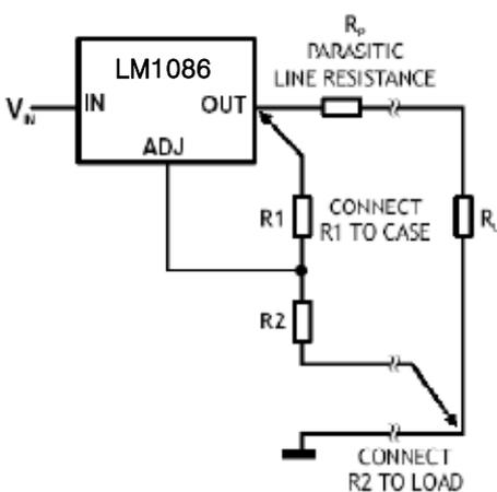
True remote sheet specification it is not possible to provide, because the LM1086 is a three terminal device.
