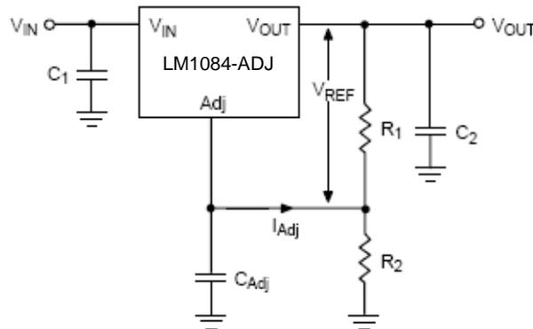
Figure 8. Resistor Divider Scheme for the Adjustable Version
