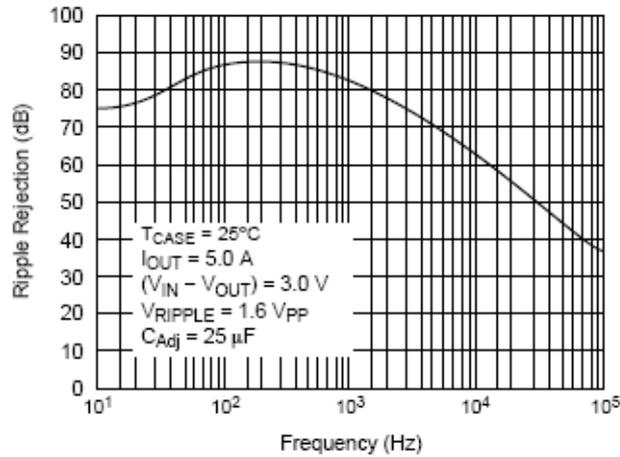
Figure 7. Ripple Rejection vs. Frequency (Adjustable Versions)
