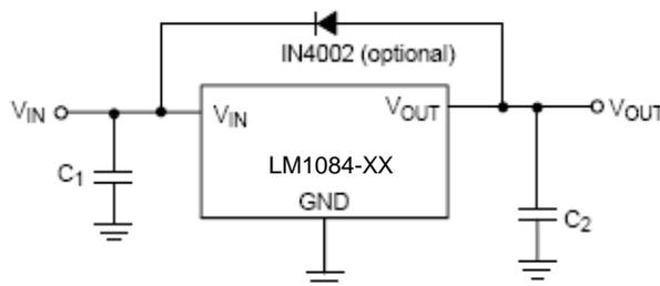
Figure 9. Protection Diode Scheme for Fixed Output Regulators
