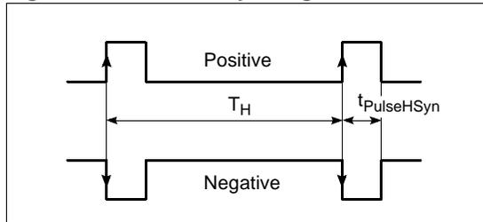
show in real time the presence or absence of the corresponding sync. signal. They are latched to 1 as soon as a single sync. pulse is detected. In order to reset them to 0 (all at once), a 1 must be written into SDetReset I<sup>2</sup>C bus bit, the reset action taking effect with ACK bit of the I<sup>2</sup>C bus transfer to the register containing the SDetReset bit. The detection circuits are then ready to capture another event (pulse). See Note 47.
