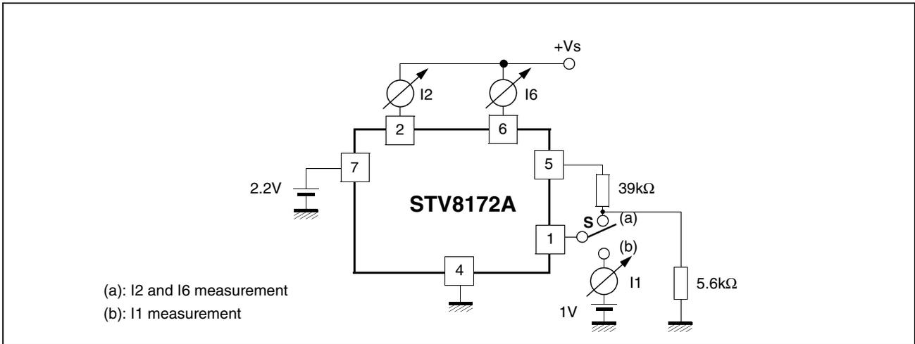
Figure 2: Measurement of  $V_{5H}$
