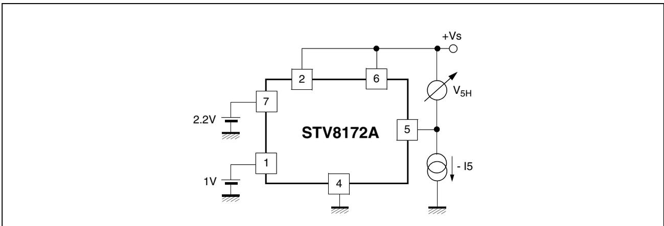
Figure 3: Measurement of  $V_{3L}$  and  $V_{5L}$
