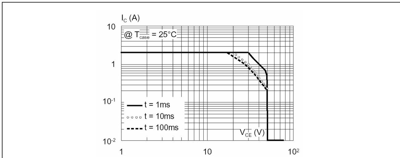
The diagram has been arbitrarily limited to max 10 (2 A).
