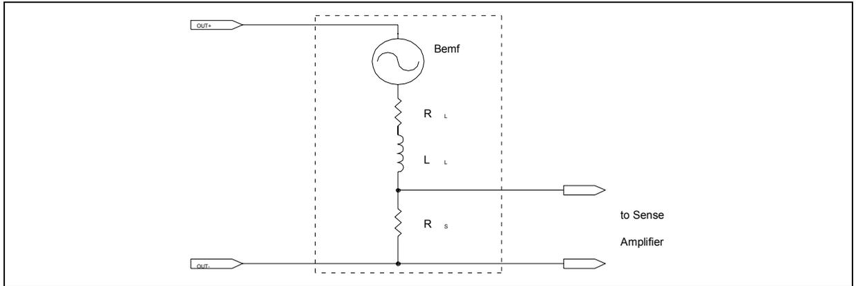
The schematic now shows the equivalent circuit of the stepper motor including a sine wave voltage generator of the Bemf. The Bemf voltage of the motor is not constant, its value changes depending on the speed of the motor.
