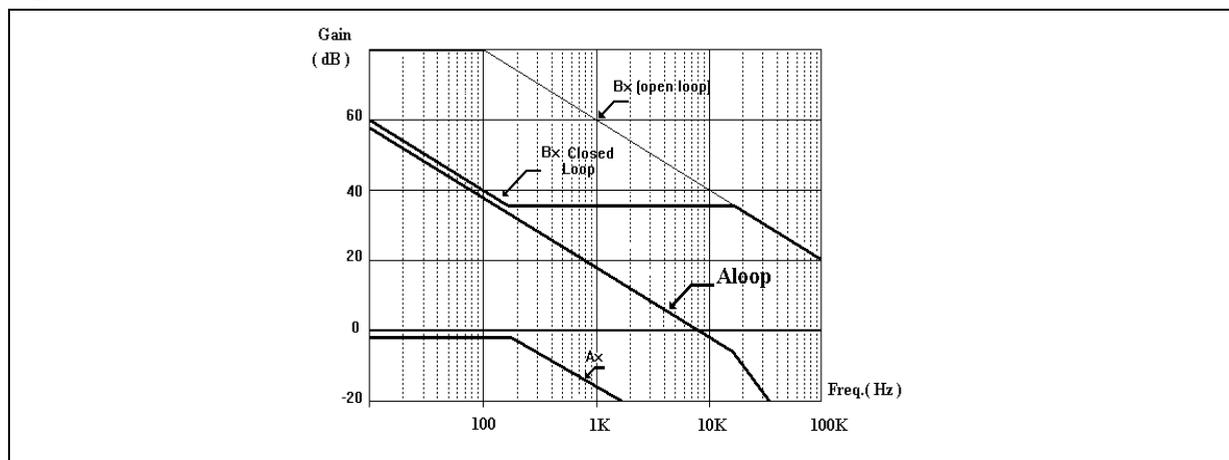
We can see that the effect of the load pole is cancelled by the zero of the Bx block ; the total Aloop cross a the 0dB axis with a slope of -20dB/decade, having in this way a stable system with an high gain at low frequency and a bandwidth of around 8KHz.
