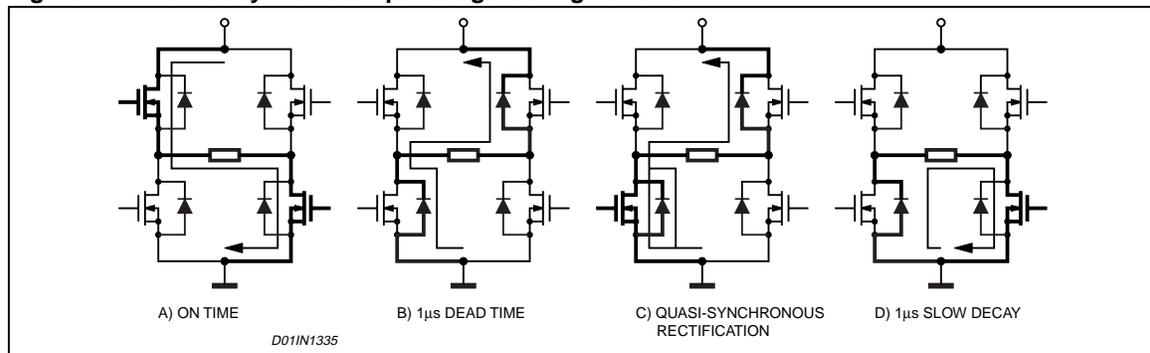
**Figure 15. Slow Decay Mode Output Stage Configurations**
