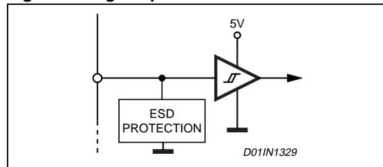
Figure 8. EN Pin Open Collector Driving
