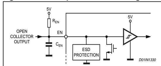
Figure 9. EN Pin Push-Pull Driving
