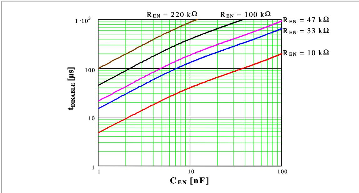
Figure 22.  $t_{\text{DELAY}}$  versus  $C_{\text{EN}}$  ( $V_{\text{DD}} = 5\text{V}$ ).
