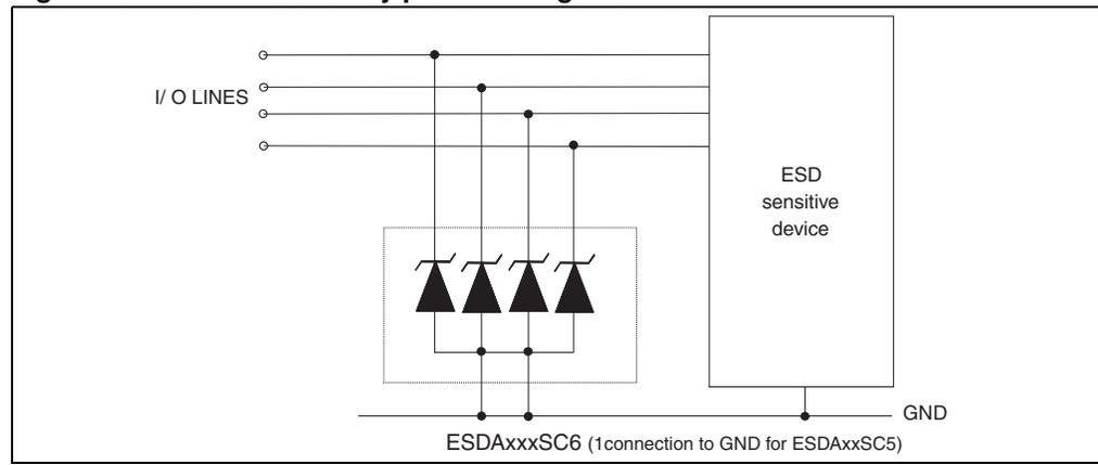
The ESDAxxSCx array is the ideal board level protection of ESD sensitive semiconductor components.
