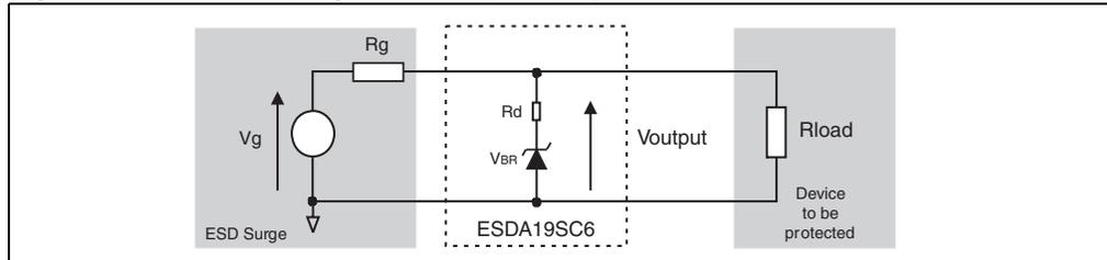
To have a good approximation of the remaining voltages at both VI/O side, we provide the typical dynamical resistance value  $R_d$ . By taking into account the following hypothesis :
