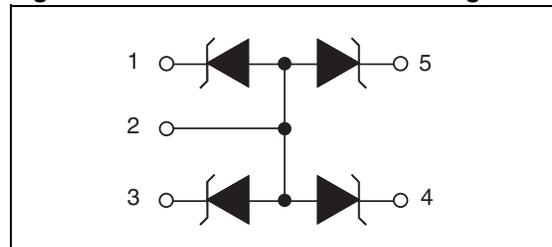
Figure 2. ESDAxxSC6 functional diagram
