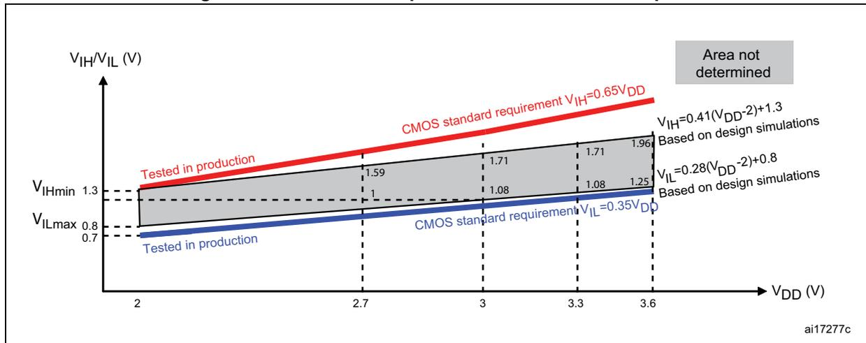
Figure 21. Standard I/O input characteristics - TTL port
