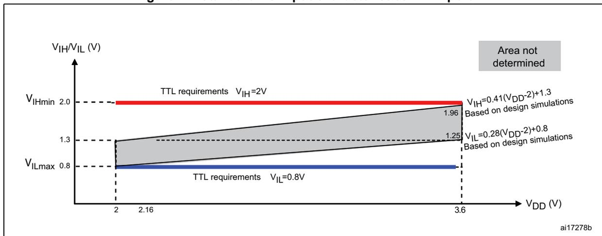
Figure 22. 5 V tolerant I/O input characteristics - CMOS port
