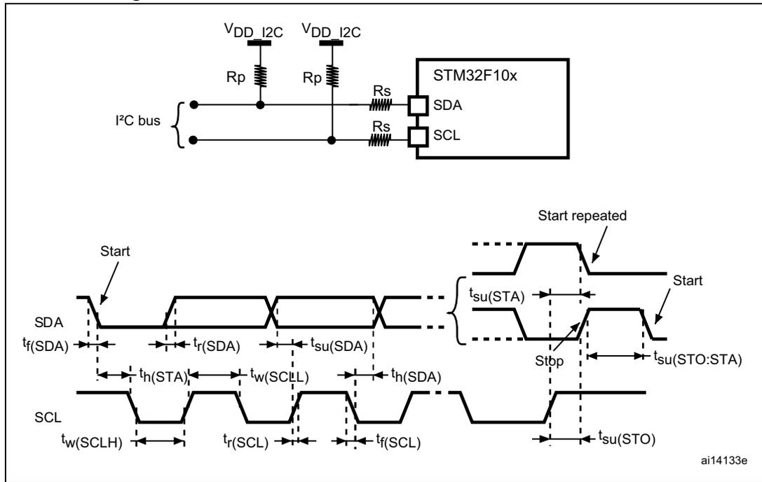
1. Measurement points are done at CMOS levels: 0.3V<sub>DD</sub> and 0.7V<sub>DD</sub>.
