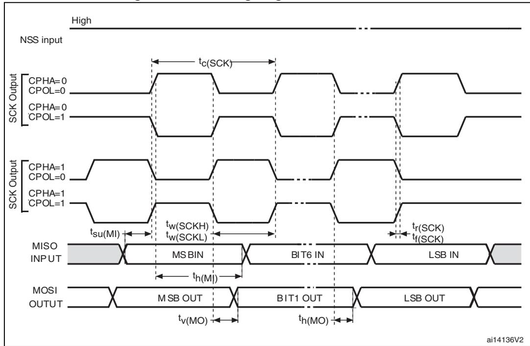
1. Measurement points are done at CMOS levels:  $0.3V_{DD}$  and  $0.7V_{DD}$ .
