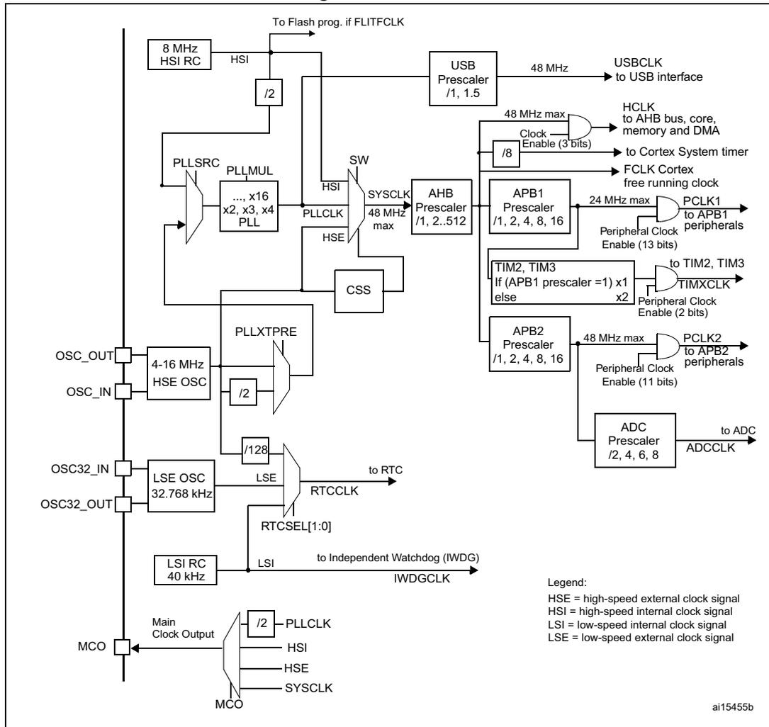
1. For the USB function to be available, both HSE and PLL must be enabled, with the USB clock output (USBCLK) at 48 MHz.
