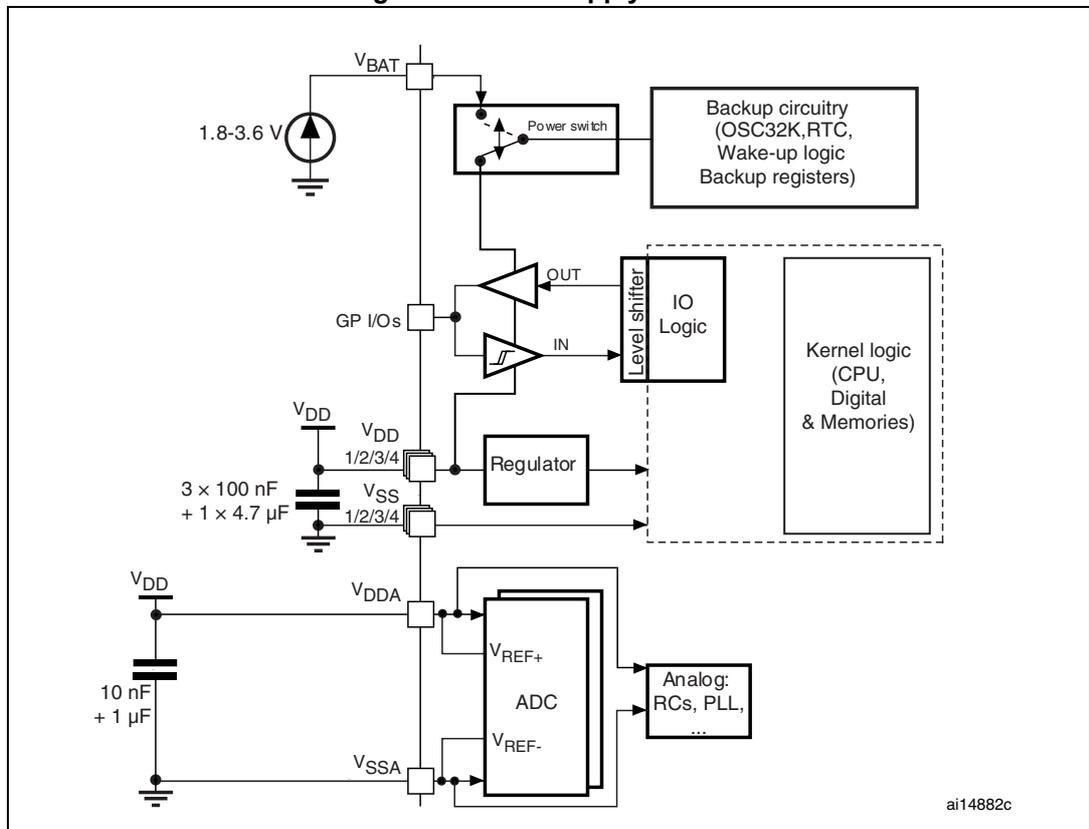
**Caution:** In [Figure 8](#), the  $4.7 \text{ }\mu\text{F}$  capacitor must be connected to  $V_{DD3}$ .
