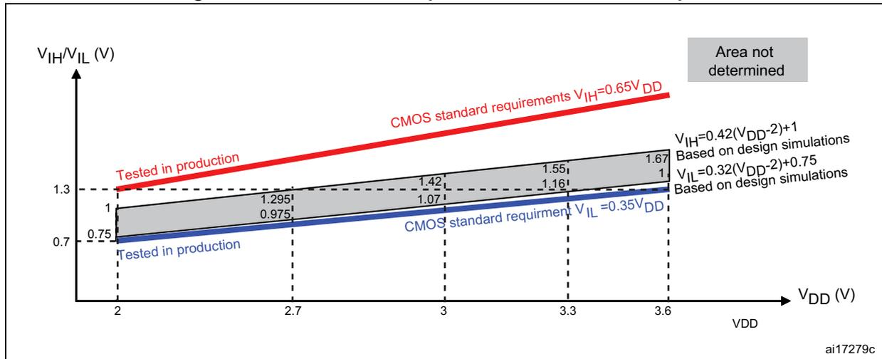
Figure 23. 5 V tolerant I/O input characteristics - TTL port
