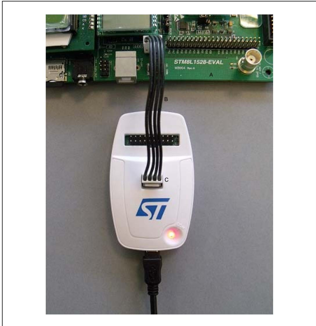
1. A = Target application board with 4-pin, 2.54 mm, low-cost connector
