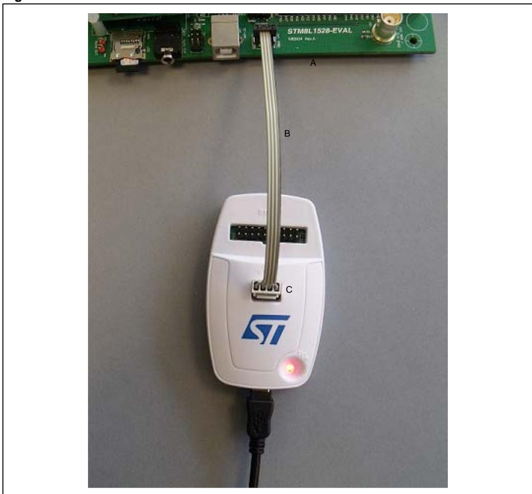
1. A = Target application board with ERNI connector
