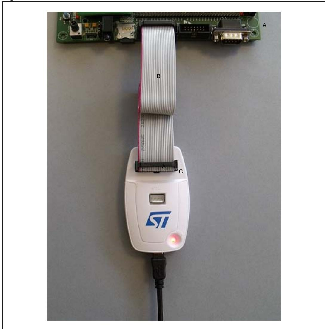
1. A = Target application board with JTAG connector
