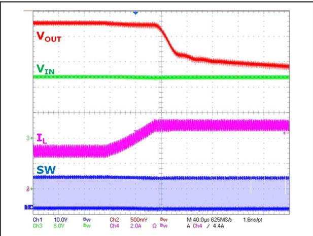
Figure 17. Short-circuit protection
