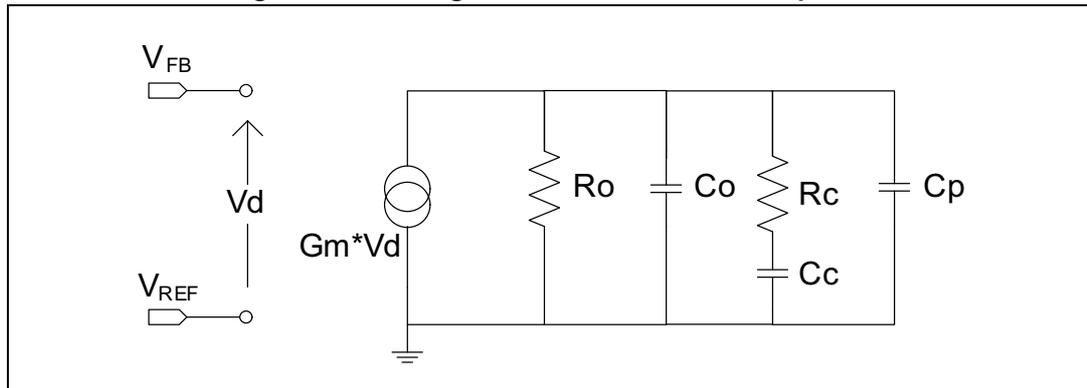
$R_c$  and  $C_c$  introduce a pole and a zero in the open loop gain.  $C_p$  does not significantly affect system stability and can be neglected.
