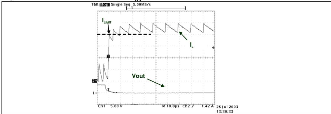
Figure 15. Short-circuit current  $V_{IN} = 30\text{ V}$
