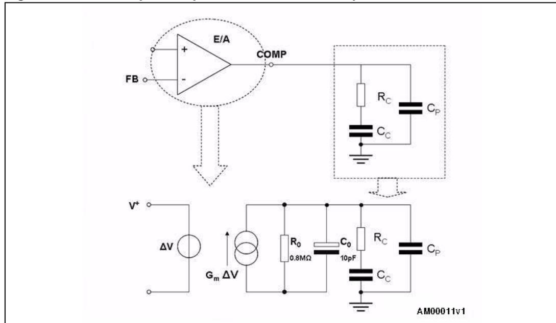
The poles of this transfer function are (if  $C_c \gg C_0 + C_P$ ):
