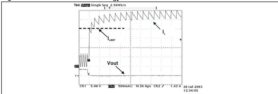
In [Figure 14](#) and [Figure 15](#), for example, it can be observed that when the input voltage increases for a given component list, the current peak increases also. The current limit is immediately triggered but the current peak increases until the current ripple during the  $T_{OFF}$  is equal to the current ripple during the  $T_{ON}$ .
