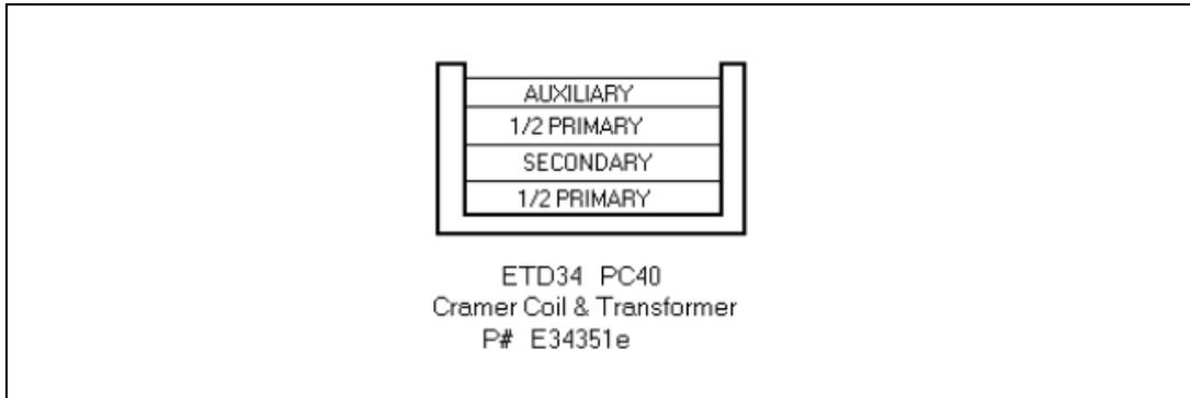
The transformer is wound with a split primary to reduce leakage inductance and minimize the snubbing needed. The auxiliary winding is placed on the outside to achieve the coupling needed for the current limiting function.
