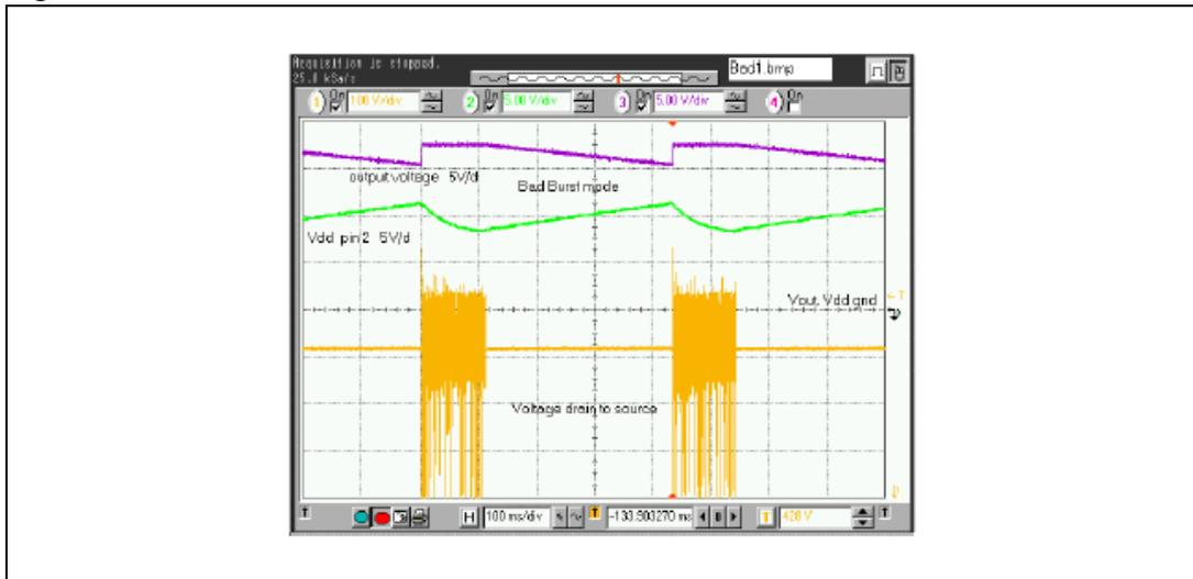
At lighter load, the  $V_{dd}$  voltage drops below the under voltage threshold, the start up circuit is reset, and the  $V_{dd}$  capacitor charges back up to the high threshold of 11 V through the start up current source.
