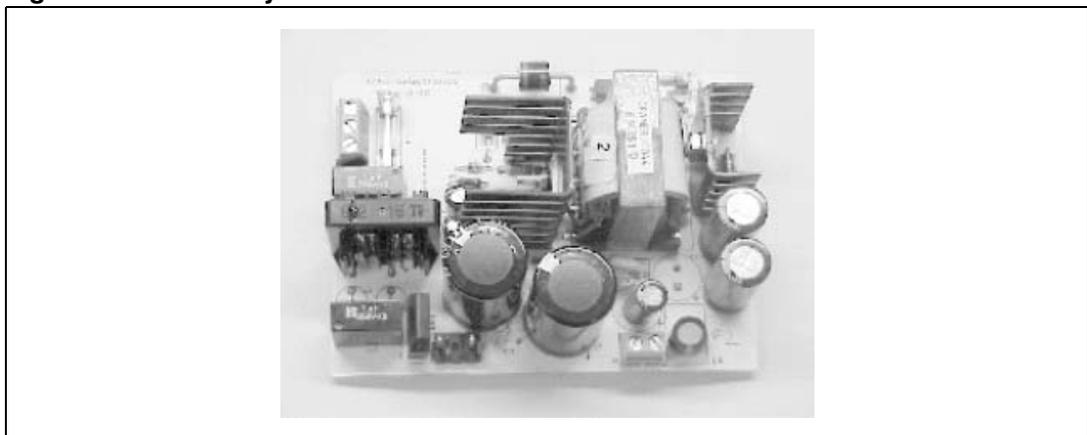
The power supply has low ripple voltage, good transient response, and be able to current limit by power limiting and cycling on and off during a hard short. One use of this application is to replace a bulky 60 Hz transformer with a lighter, better regulated, more efficient alternative for an audio or entertainment system.
