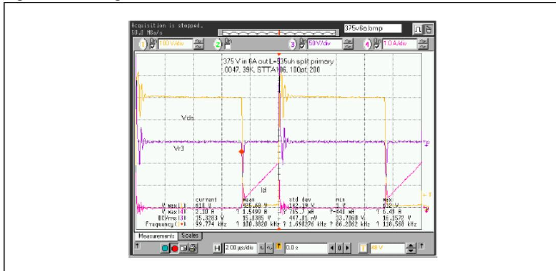
Figure 5 illustrates the voltage drain to source, and the current through the VIPer100A-E.
