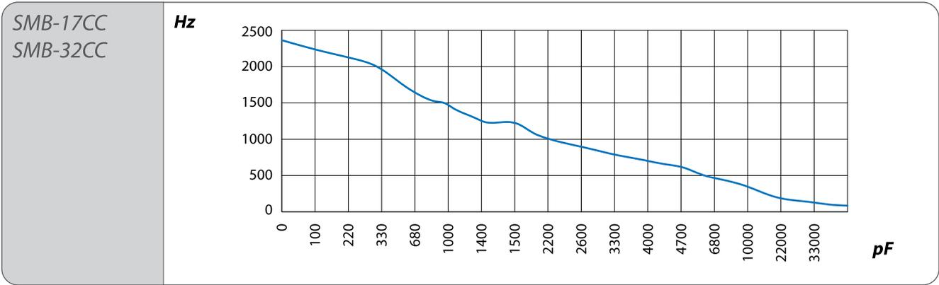
**Sound pressure level vs. external capacitor (c)**
