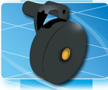
The SAST-2155 is a transducer version of the SAS-2155-S. The drive electronics are not included on the internal pcb and must be created by the customer to realize a good functional sound output. The maximum dB(A) level is obtained if the drive frequency is used between 2kHz and 3kHz. Several signals can be combined or produced in continuous, intermittent, warbler or sweep mode. Square wave signals give extra sound dimensions because of their harmonic content.
