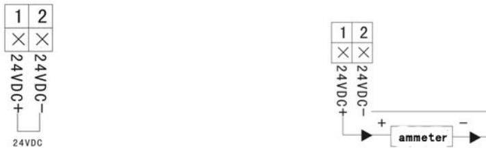
Wiring diagram of integral explosive-proof two wire
