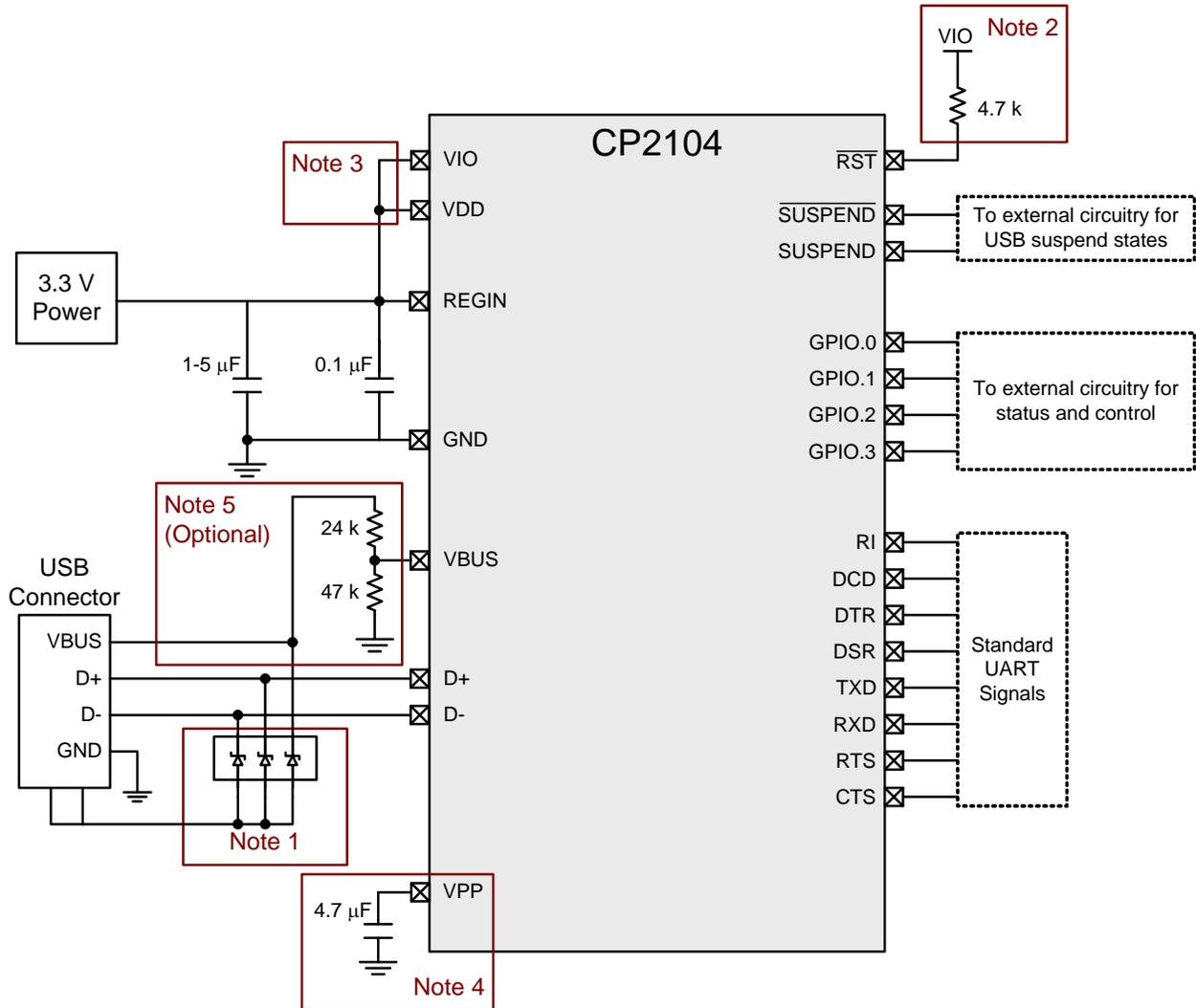
**Note 1 :** Avalanche transient voltage suppression diodes compatible with Full-speed USB should be added at the connector for ESD protection. Use Littelfuse p/n SP0503BAHT or equivalent.
