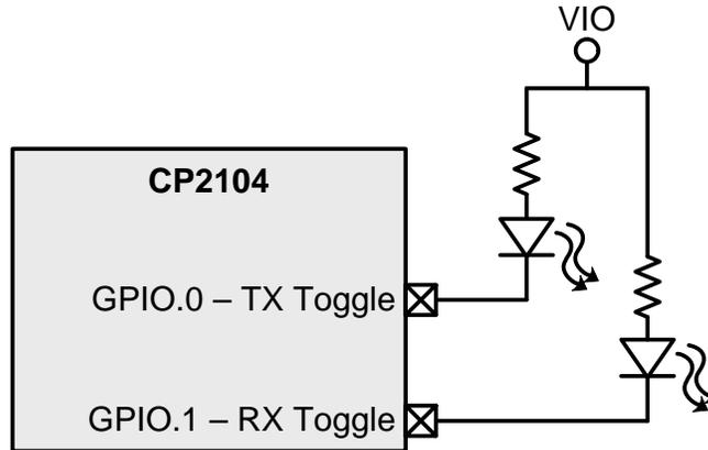
Figure 5. Transmit and Receive Toggle Typical Connection Diagram
