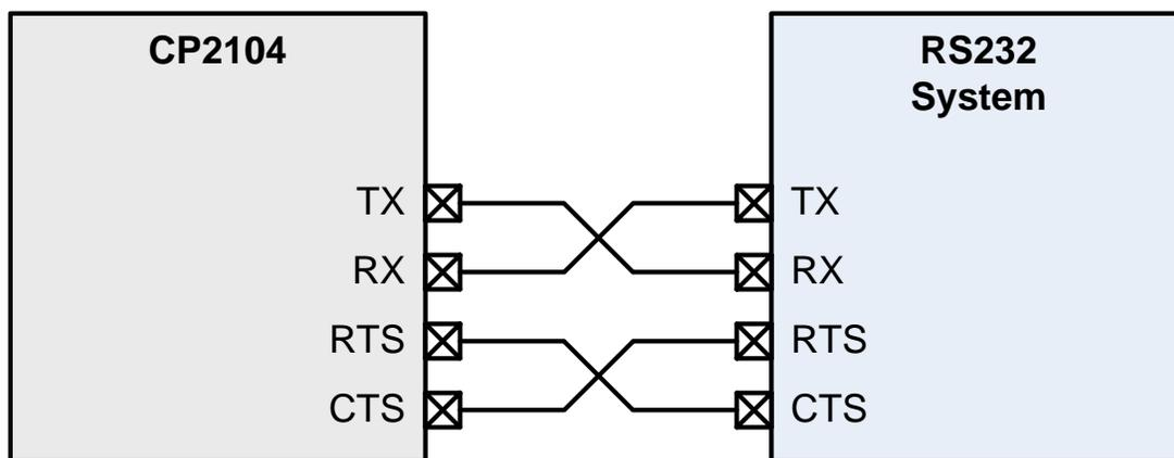
Figure 7. Hardware Flow Control Typical Connection Diagram
