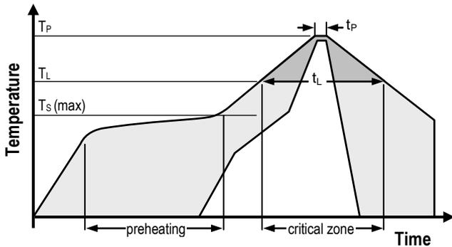
**Figure 7** Soldering profile according to JEDEC standard.  $T_P \leq 260^\circ\text{C}$  and  $t_P < 30\text{sec}$  for Pb-free assembly.  $T_L < 220^\circ\text{C}$  and  $t_L < 150\text{sec}$ . Ramp-up/down speeds shall be  $< 5^\circ\text{C}/\text{sec}$ .
