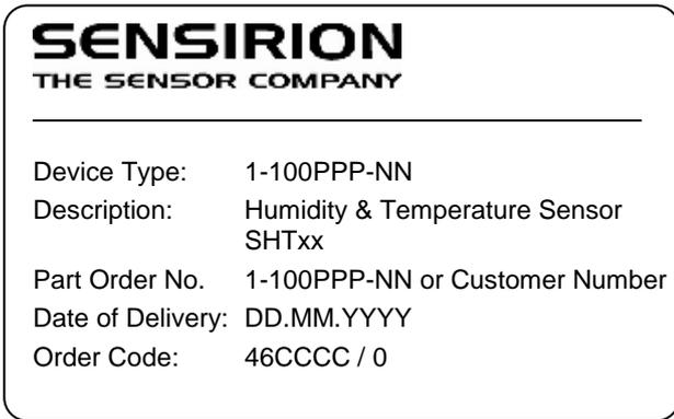
**Figure 13:** Second label on reel: For Device Type and Part Order Number (See Packaging Information on page 2), Delivery Date (also Date Code) is date of packaging of sensors (DD = day, MM = month, YYYY = year), CCCC = Sensirion order number.
