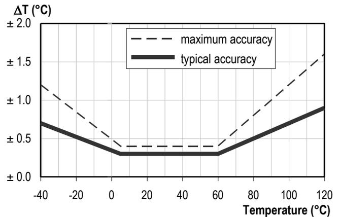
**Figure 3** Typical and maximal temperature accuracy tolerance
