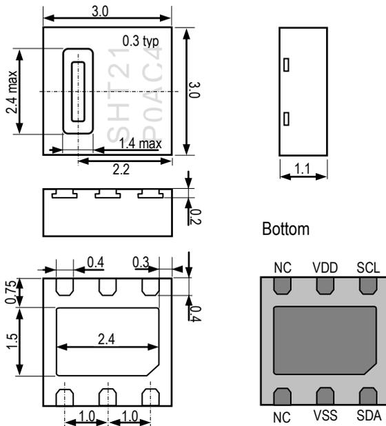
**Figure 1:** Drawing of SHT21P sensor package, dimensions are given in mm (1mm = 0.039inch), tolerances are  $\pm 0.1$ mm. The die pad (center pad) is internally connected to VSS. The NC pads must be left floating. Numbering of E/O pads starts at lower right corner (indicated by notch in die pad) and goes clockwise (compare Table 2).
